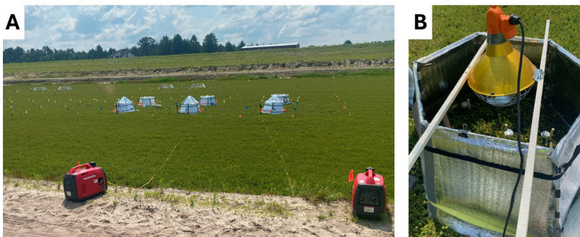
Figure 4. Set up of the acute heat stress experiments. A. OTCs covered with insulation blankets. The first row of three OTCs includes patio lamps to induce a “pulse” of heat stress for two hours. The second row consists of control OTCs without lamps. Generators were used to power the patio lamps. B. Close-up of the OTC with a patio lamp on top. Canopy and fruit temperature sensors, as well as relative humidity sensors were installed.
