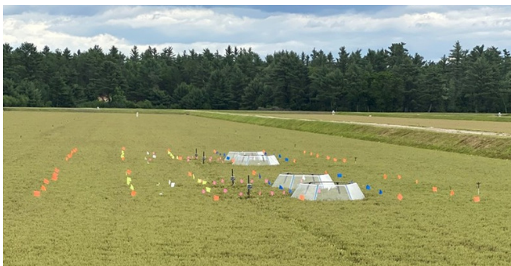
Figure 2. Open-top chambers (OTCs) and control plots established to study the effect of long-term heat stress on cranberry fruit rot.
