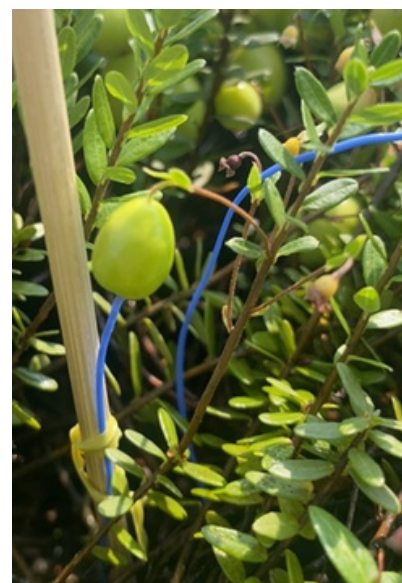
Figure 3. Micro-thermocouple inserted into growing fruit to monitor internal fruit temperature during heat stress experiments. The micro-thermocouple was inserted through the calyx, 3 mm inside the fruit.
